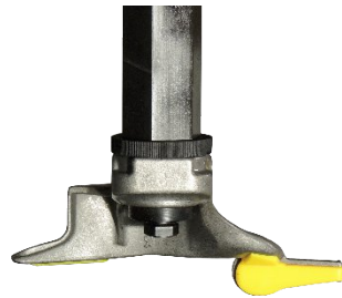
Plastic Demount Head Clamps for added Wheel Protection
